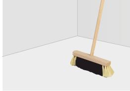
**Step 2:** Ensure the sub-floor is solid level, clean and dust free. Wooden floors can be reinforced with ply board or suitable tile backer board.
